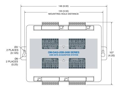
Figure 3-7. OM-DAQ-USB-2401 Wall Mounting Dimensions
